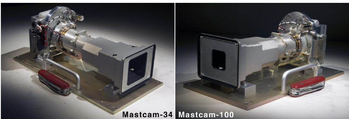
Figure 28. Fixed-focal length (FFL) Mastcams. The only distinguishing difference in outward appearance between the cameras is the aperture size in the front baffle.
