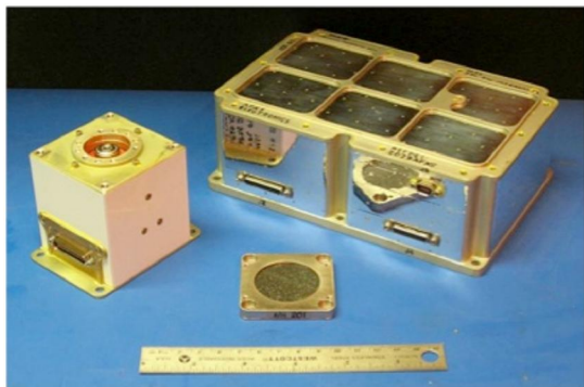
Figure 10. APXS hardware: sensor head (left), electronics unit (right), and calibration target (middle front).
