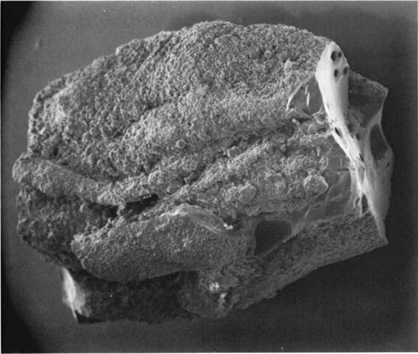
4.10 Ropy glass fragment, 1 mm long, of KREEP glass (12033). (NASA S.70 17107. Courtesy D. S. McKay.)
